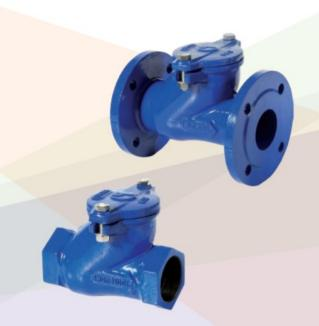
The series 07 valves are ball check valves made of ductile iron with NBR coated ball and seals and S/S bolts. Available in DN32,40,50 and 80 threaded and DN80, 100 and 150 flanged.
